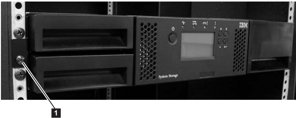
Figure 1-10. Securing the 2U library to the rack
