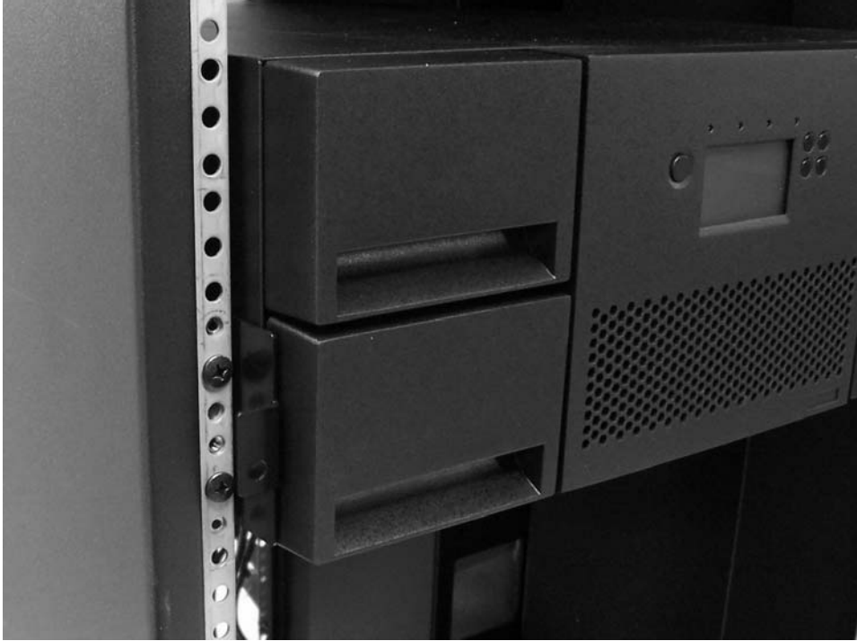
Figure 1-9. Sliding the 4U library into the rack
