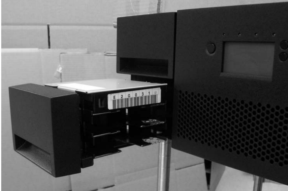
Figure 1-32. 4U library I/O Station in the lower left magazine
