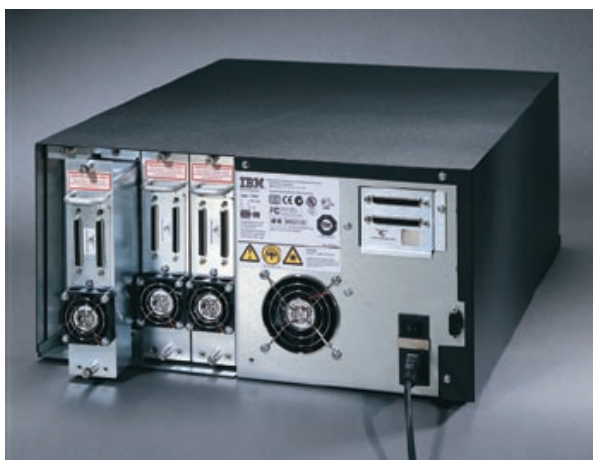
Rear view of 7334 Model 410 8 mm Tape Library showing user-installable tape drives
