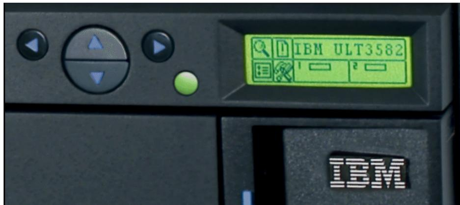
Figure 6-4 IBM 3582 operator panel
