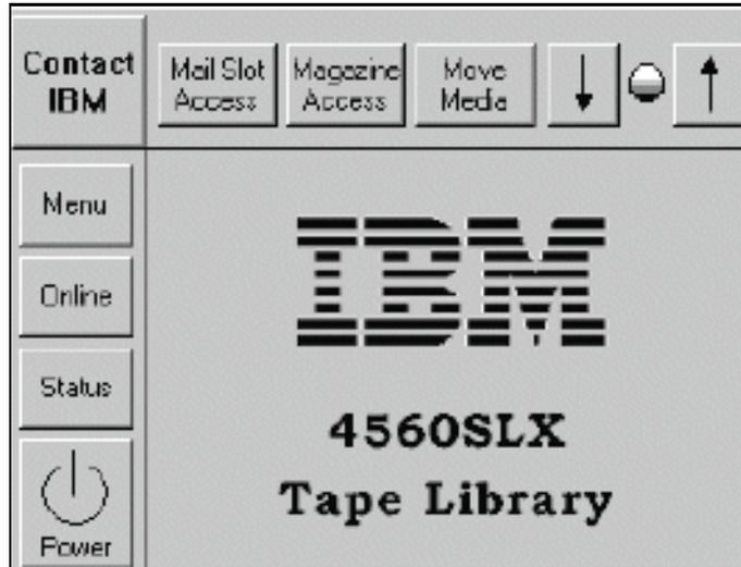
Figure 9-4 4560-SLX touch screen front panel
