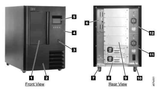
Figure 1. Tape Library Subsystem (Stand-Alone Configuration)
