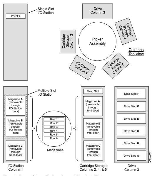
Figure 2. Storage Column Configurations and Coordinate System
