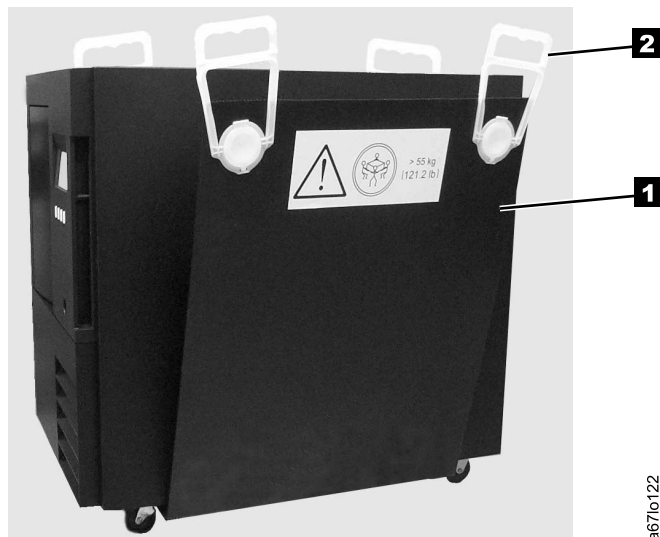
Figure 9. The sling for lifting the 3583 Tape Library
