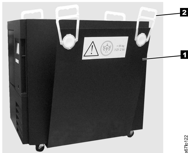
Figure 12. The sling for lifting the 3583 Tape Library
