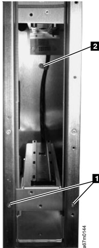
Figure 7-27. Removing the Lower Fibre Channel Bracket Sub-Assembly
