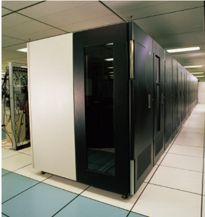
A 16-frame IBM TotalStorage Enterprise Tape Library 3494 high availability configuration with two service bay frames
