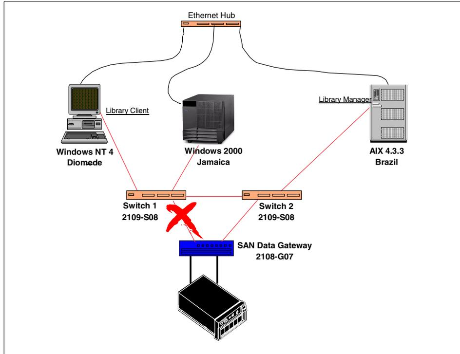
Figure 121. Link failure test setup
