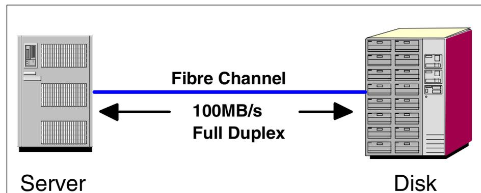
Figure 1. Point-to-point Fibre Channel connection
