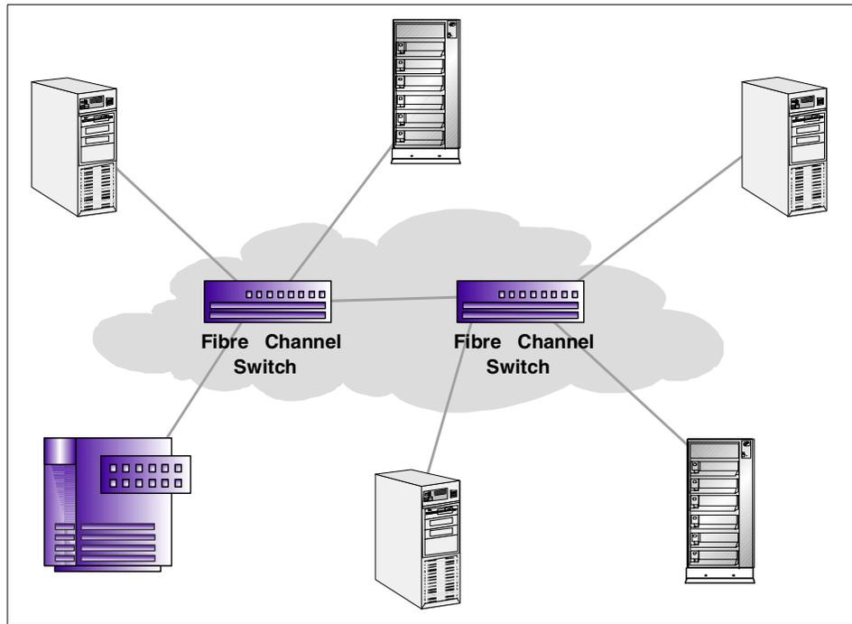
*Figure 3. Non-cascaded switched fabric*
