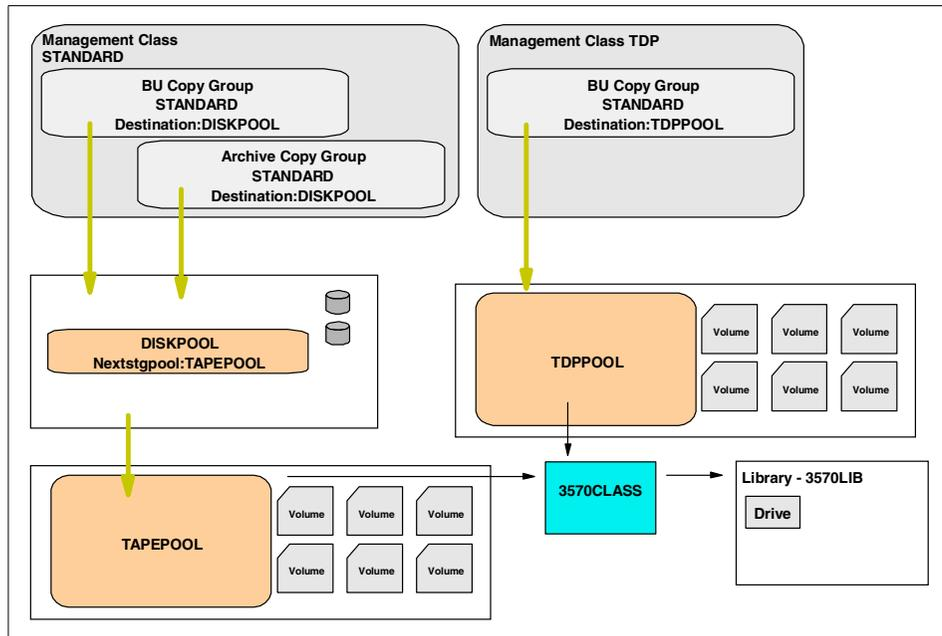
Figure 98. Storage setup for the AIX server
