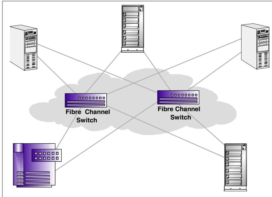
Figure 4. Cascaded switched fabric
