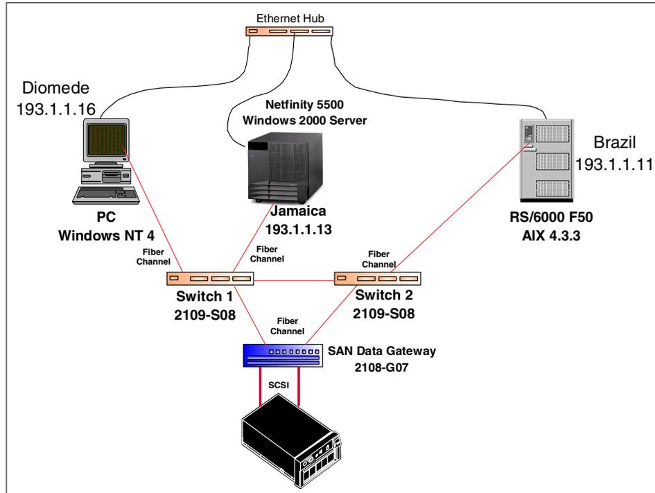
Figure 39. Using IBM SAN Fibre Channel Switch
