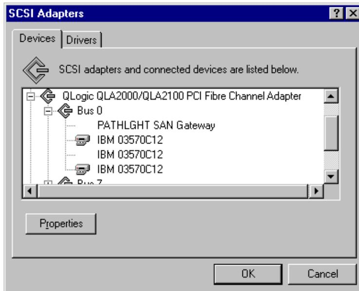
Figure 47. Qlogic device driver configuration, devices visible to HBA
