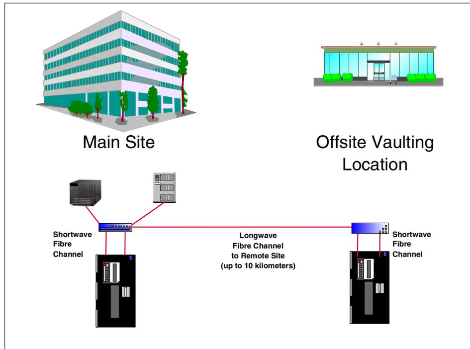
Figure 16. Remotely connected tape library
