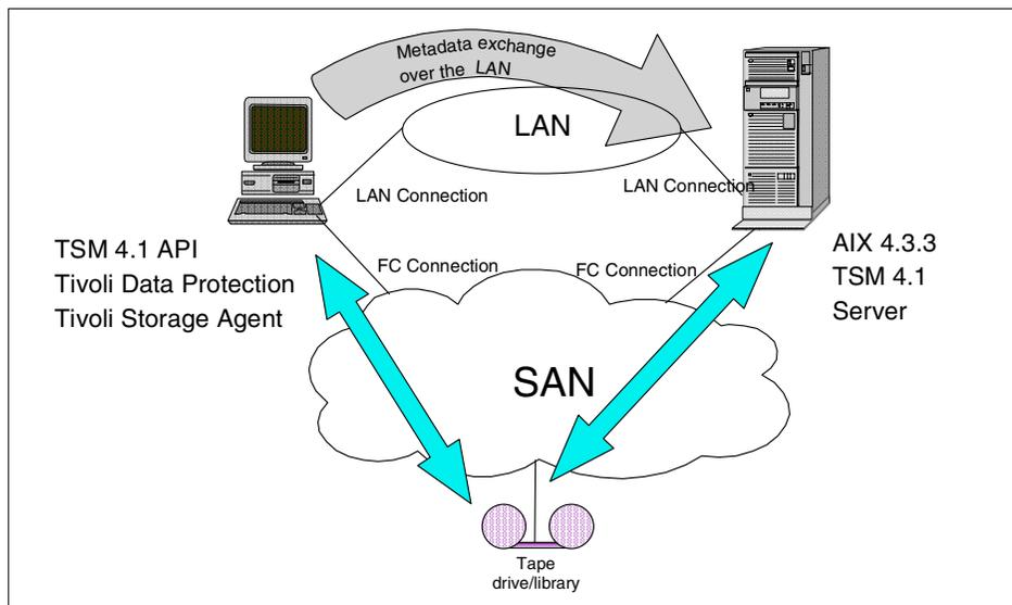
Figure 44. TSM LAN-free storage solution
