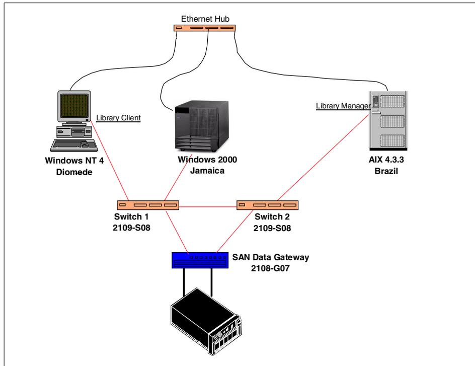
Figure 115. Cascading switches setup
