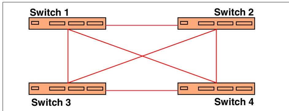
Figure 17. Meshed switch topology
