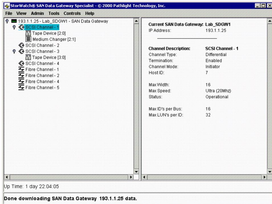
Figure 129. Devices attached to the gateway
