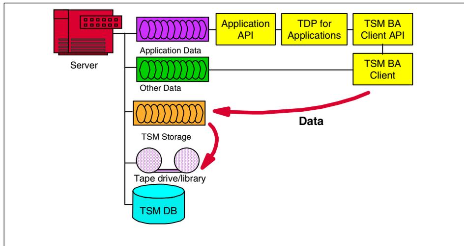
Figure 89. Application server and TSM server on one machine
