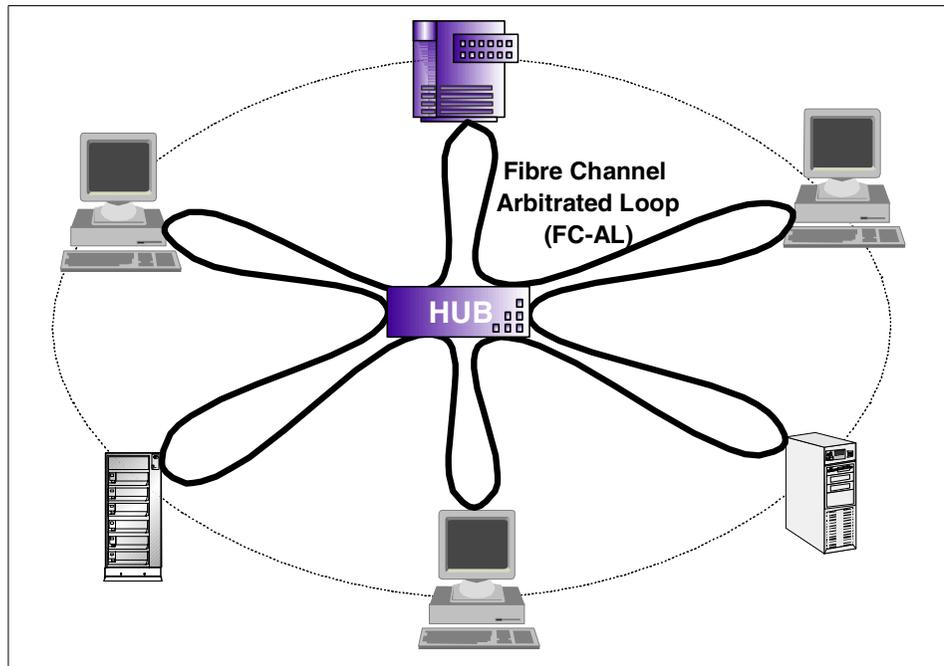
Figure 2. Fibre Channel arbitrated loop (FC-AL)
