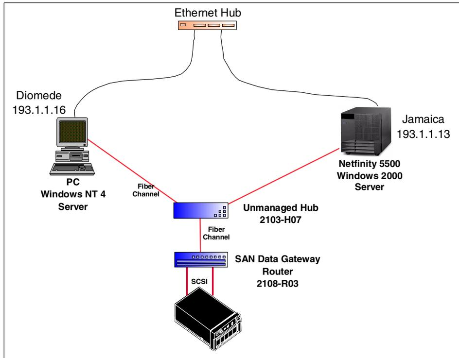
Figure 37. Using IBM SAN Data Gateway Router and Hub
