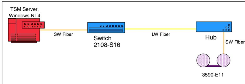
Figure 111. Distant connection of a 3590 FC attached tape device
