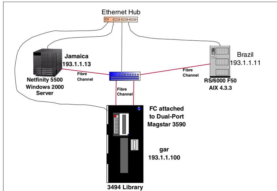
Figure 42. Lab setup for IBM 3494 partitioning
