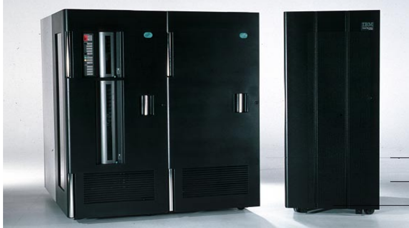
Figure 4-16 IBM VTS along with 3494 tape library
