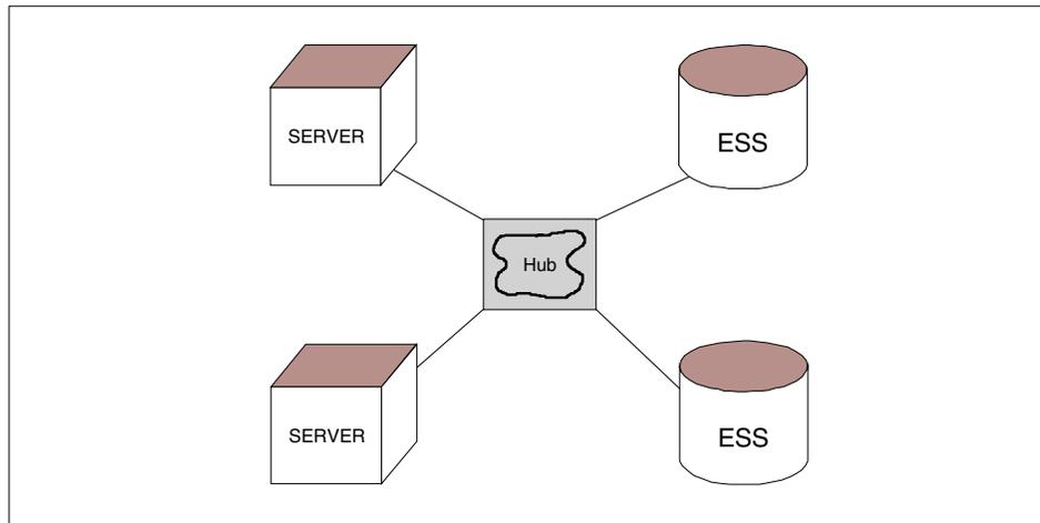
Figure 8. An example of arbitrated loop with a hub
