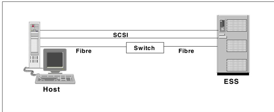
Figure 37. SCSI setup between the NT host and ESS
