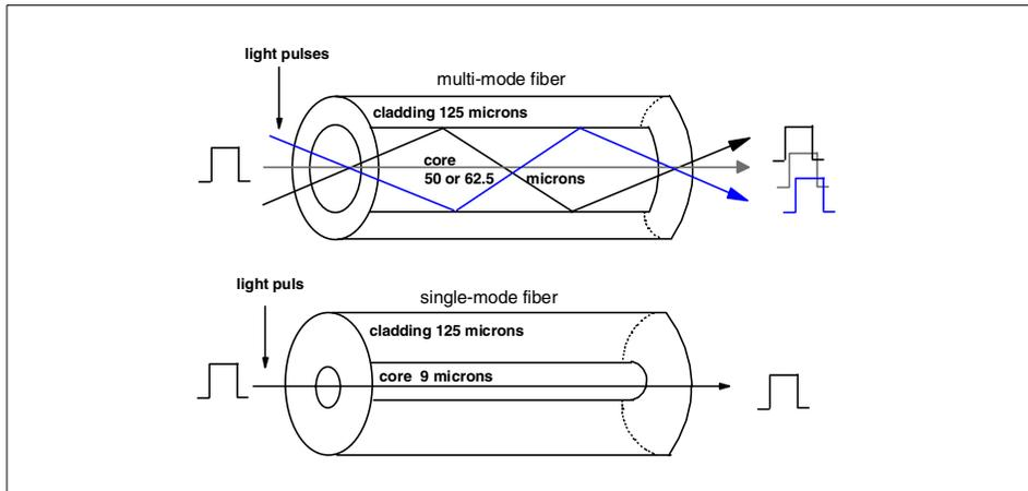
Figure 1. Light propagation through multi-mode and single-mode fiber
