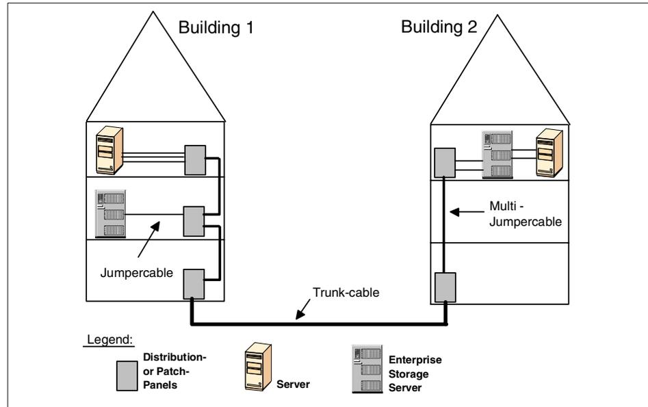
Figure 4. An example of fiber cabling infrastructure
