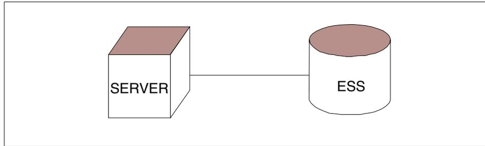
Figure 5. An example of point-to-point topology
