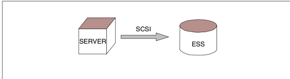
Figure 32. SCSI connection — server to ESS
