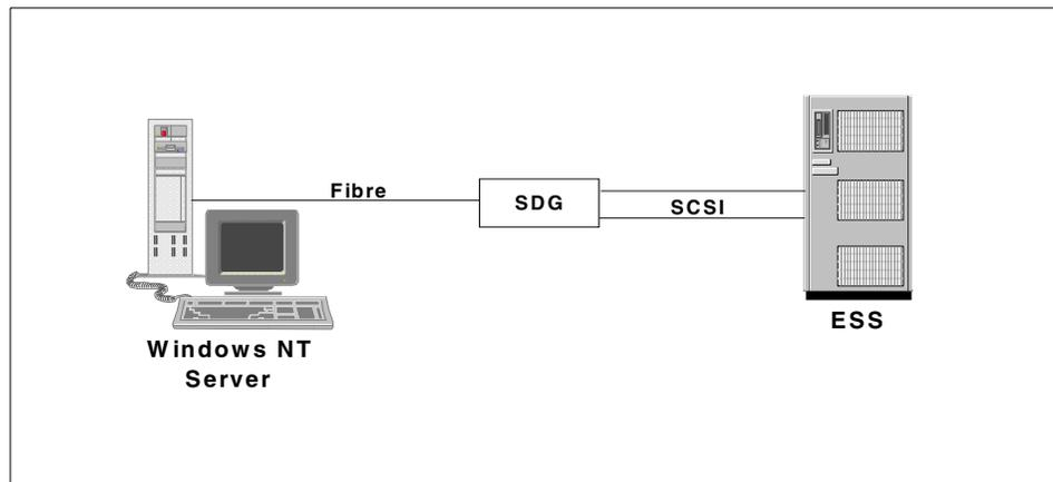
Figure 61. System setup for SDG to FC migration
