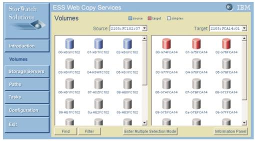
Figure 52. Volumes panel with source and target pairs selected
