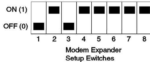
Figure 248. Modem Expander Setup Switch Settings (S007455I)
