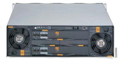
The 3U DS6000 expansion enclosure can be mounted in a standard 19-inch rack. The front of the enclosure contains the docking sites where you can install up to 16 DDMs. The DDMs are installed in a horizontal position with a locking handle. The rear of the enclosure provides the docking sites for the power supplies and the controller cards.
