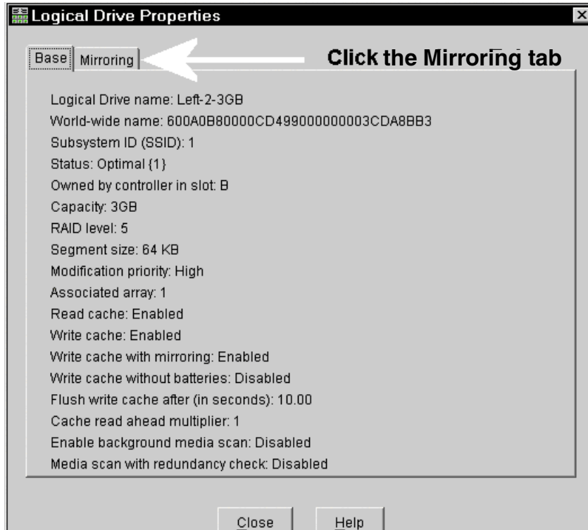
Figure 6-25 Base drive properties
