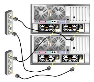
2. Power on the engine by pressing the power control button on the front of the engine. (Note the order in which you start the engines. You must shut them down in the reverse order.)
