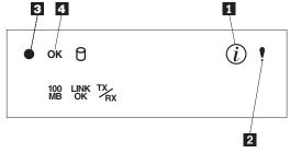
Information LED 2 System error LED Power-on LED
