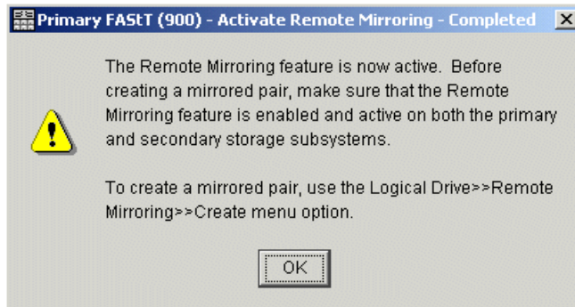
Figure 8-15 Activate Remote Mirroring Wizard - Completed
