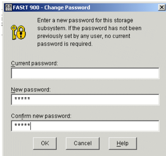
Figure 5-22 Setting a password on the FAST Storage Server
