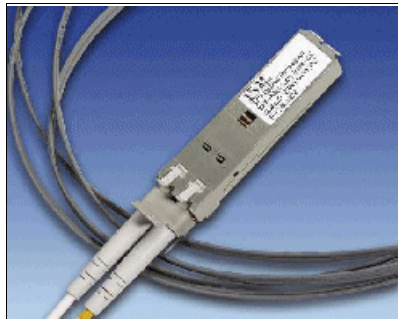
Figure 2-2 Small Form Pluggable (SFP) with LC connector Fibre Cable
