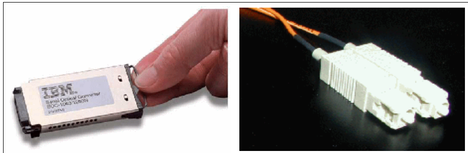
Figure 2-4 GBIC Connector and SC Fibre Connection
