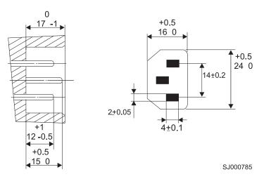
Figure 31. PDU cable that is shipped with the 2005 Model H08 and Model H16
