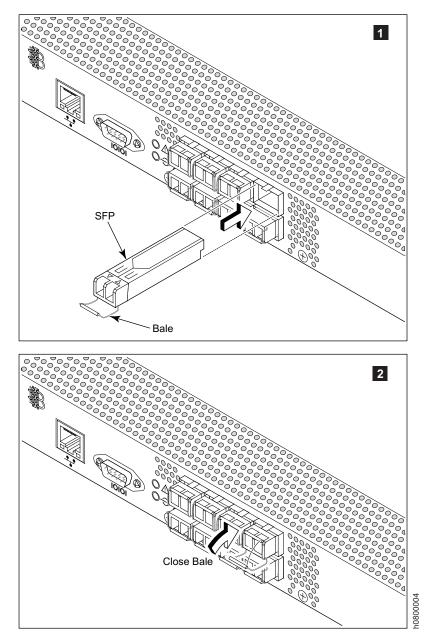
Figure 17. Installing an SFP
