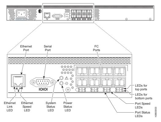
Figure 16. Detailed view of the Model H08 LEDs
