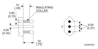
Figure 25. Power cable for Italy
