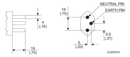
Figure 27. Power cable for Switzerland
