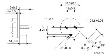
Figure 22. Power cable for Denmark
