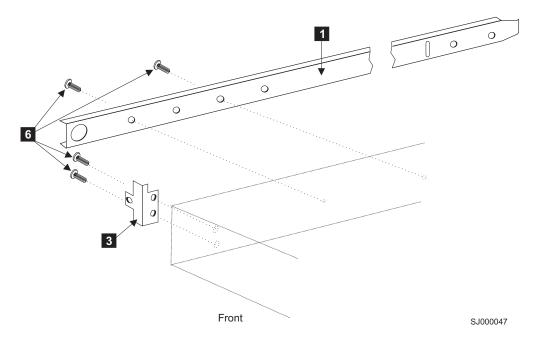
Figure 11. Mounting the moving portion of the slide and mounting brackets to the switch
