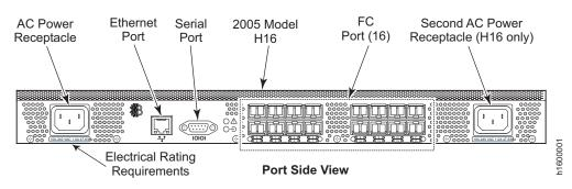
Figure 7. Port side of the Model H16
