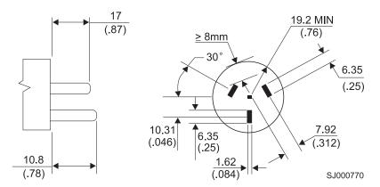
Figure 19. Power cable for Australia
