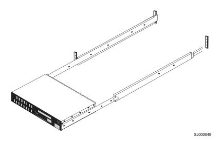
Figure 13. Inserting slides into the rack rails
