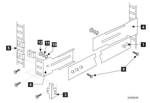
Figure 12. Mounting the fixed portion of the rail and the locking ears to the rack
