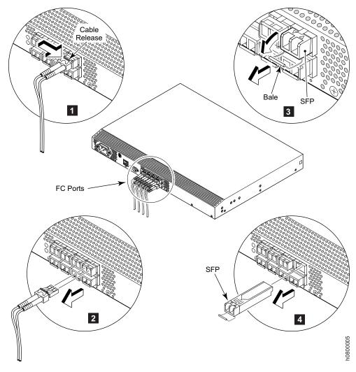
Figure 18. Removing an SFP
