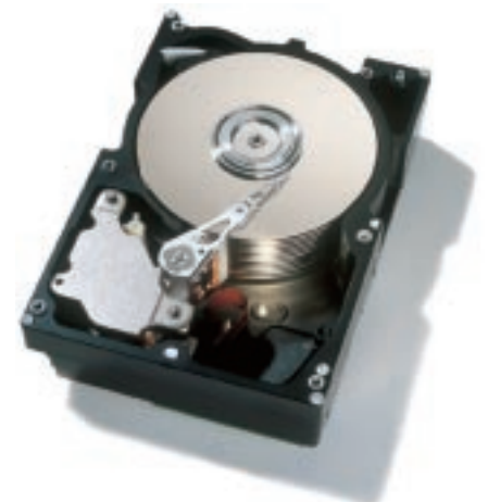
Ultrastar 18ZX 3.5-inch 18.2 GB high-performance disk drive
