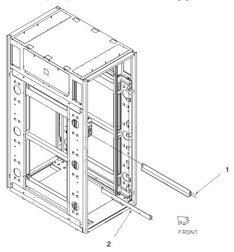
Install the nut clip in the middle of the fourth EIA unit above where you installed the drawer rails, as shown in the following figure:
