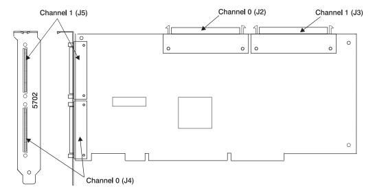
This adapter might be preinstalled in a hot-swap carrier for use in certain system types. This carrier allows the adapter to be installed and removed without removing the top cover of the system in which it is installed. Refer to the adapter installation and removal procedures located in your system's user or service guide.
