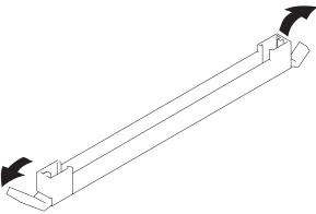
5. The memory modules are keyed so that they can only be inserted one way. Align the memory module notches with the keys in the memory connector.
