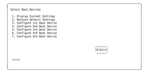
Display Current Settings: Lists the current order of devices in the boot list. The following screen shows an example of this display.
