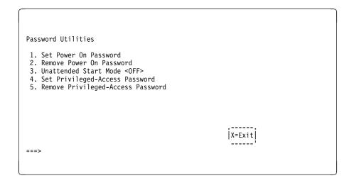
**Set Power On Password:** Setting a power-on password helps protect information stored in your server. You can use any combination of up to eight characters (A-Z, a-z, and 0-9) for your password. The password you type is not displayed on the screen. Press Enter when you are finished; you must type the password again for verification.
