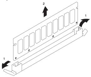
5. Store any memory modules you are no longer using in a static-protective package. Make a note of the memory module size and speed for future reference.
