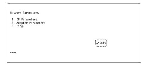
Selecting the IP Parameters option displays the following screen:
