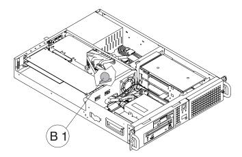
2. Remove the battery as shown in the following figure. To replace the battery, reverse the motions.
