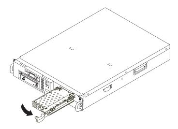
**Note:** It is important to ensure that the drive carrier is inserted firmly into the connector located in the rear of the bay.
