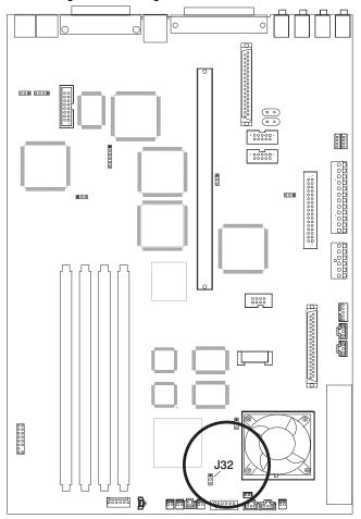
2. Remove any adapters that are blocking the jumper.
