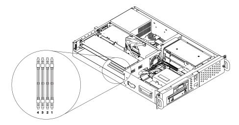
2. Remove any adapters that are blocking the memory module connectors (see "Removing Adapters" on page 4-26).
