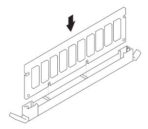
Attention: Inserting the memory module at an angle may cause damage.
