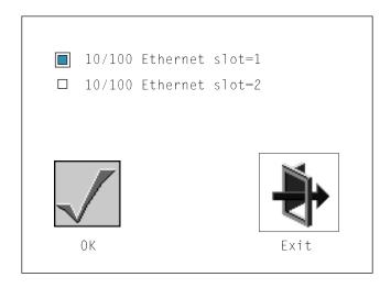
The next screen allows you to select the type of adapter you have just chosen (or allow the system to select the type automatically). Use the arrow keys or mouse to highlight a selection. To choose the highlighted selection, press the spacebar, then highlight the **OK** icon and press Enter.
