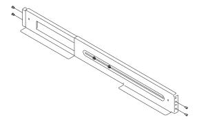
3. Install the two rack mount brackets. Place one bracket over the left rail pin guides, then install the screw between the rail alignment pins. Install the second bracket over the right rail pins in the same manner.
