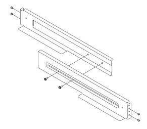
2. Select the correct size of alignment pins for your specific rack. Install the rails into the rack by screwing two pins into the front of each rail, installing one in the lower rail hole and one in the third hole from the bottom as shown in the diagram. Screw two pins into the back of each rail in the same manner.
