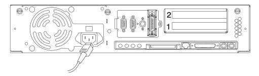
2. Plug these power cables into electrical outlets.
