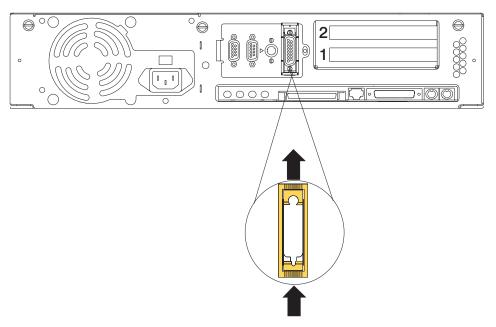
3. The thick Ethernet cable is now installed.
