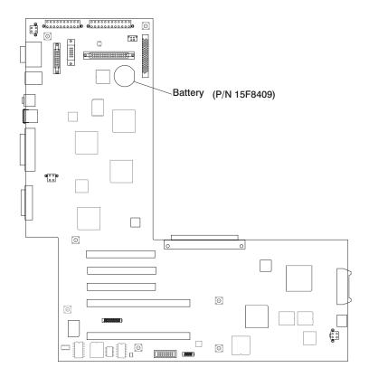
6. If needed, remove any adapters mounted in the top two adapter slots as described in "Removal of Adapters" on page 246.
