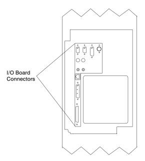
14. Remove the screws that secure the I/O board to the system unit.
