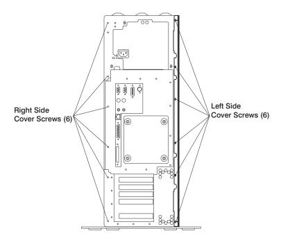
Note: The left and right side covers are interchangable, but should not be switched because the left side cover contains a reference diagram.
