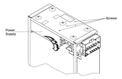
**Attention:** When you remove the power supply, ensure that the power supply does not drop down and damage the I/O board components or connectors.
