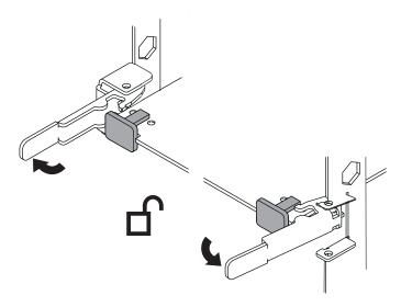
6. Remove the card from the connector. Be sure to store the processor card in a safe place.
