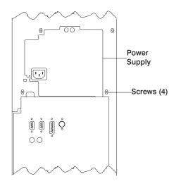
Remove the retaining screws that secure the power supply to the top of the system unit.
