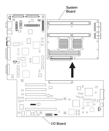
14. Carefully remove the system board from the system unit.
