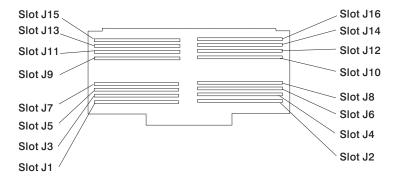
Note: Memory modules must be installed in pairs and in the correct slot configuration. (Slots J1 and J2, J3 and J4, J5 and J6, and so on.)
