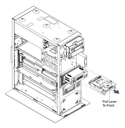
**Note:** On a new hard drive, pull the lever to the front before installing. Ignore the arrow printed on the top of the lever that points to the right.
