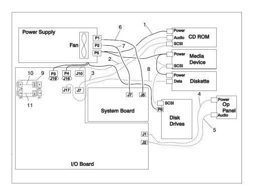
Note: P3 cable goes into designated socket J19, and P4 cable goes into designated socket J16.
