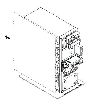
5. To remove the top cover, remove the screw at the front and the three screws at the rear and lift the cover off. (The side covers must have been removed previously.)
