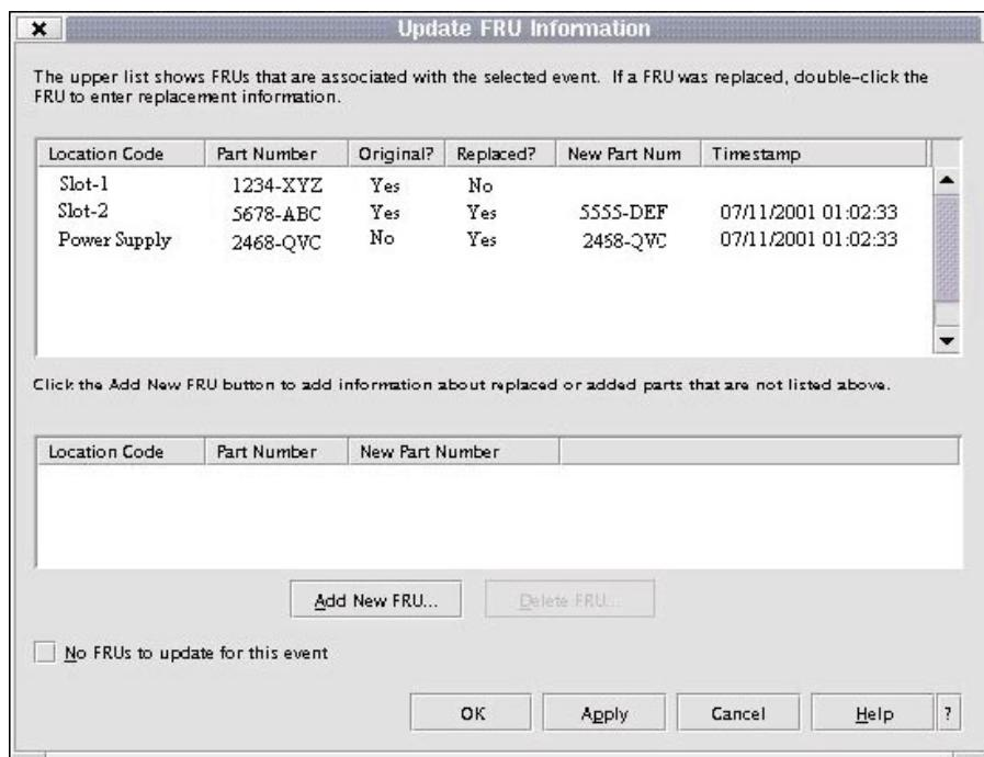
In this example, three parts are involved in this serviceable event. The system recommended that the part in Slot-1 be changed (Original=Yes), but the representative decided not to change the part. The HMC also recommended that the part in Slot-2 be changed, and the part was replaced by a part, although one with a different part number. The part in PowerSupply was not in the initial recommendation for replacement, but was replaced with a part with the same part number.
