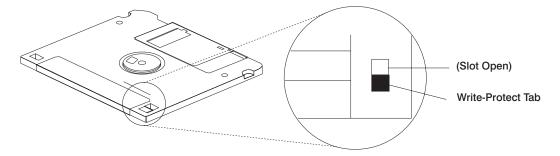
To allow writing onto a diskette, slide the write-protect tab to cover the protect slot, as shown in the illustration.
