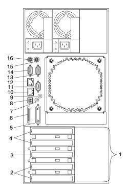
PCI slots 1-2 1 PCI slots 1-5 2 64-bit/3.3V 3 PCI slot 3 PCI slots 4-5 64-bit/5V 32-bit/3.3V 5 Parallel connector 6 SCSI connector 7 Attention LED 8 Rack indicator connector Power LED 9 10 Ethernet connector 2 11 Serial connector 1 12 Ethernet connector 1 13 Serial connector 3 14 Serial connector 2 15 Mouse connector 16 Keyboard connector
