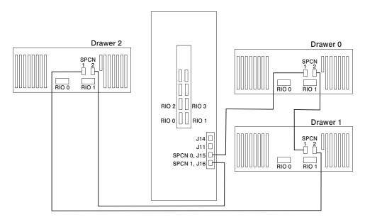
System Rack Attached to Four I/O Drawers
