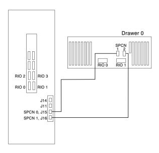
System Rack Attached to Two I/O Drawers
