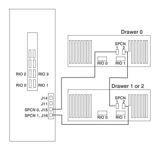
System Rack Attached to Three I/O Drawers
