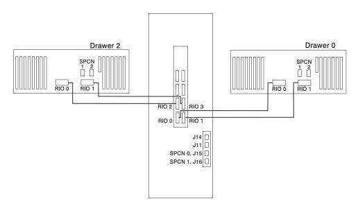
System Rack Attached to Three I/O Drawers
