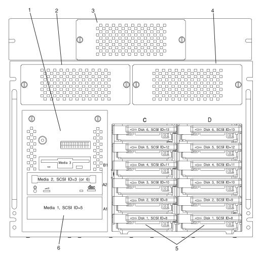
**Note:** The SCSI IDs shown for media devices indicate how these devices are set when shipped from the factory.
