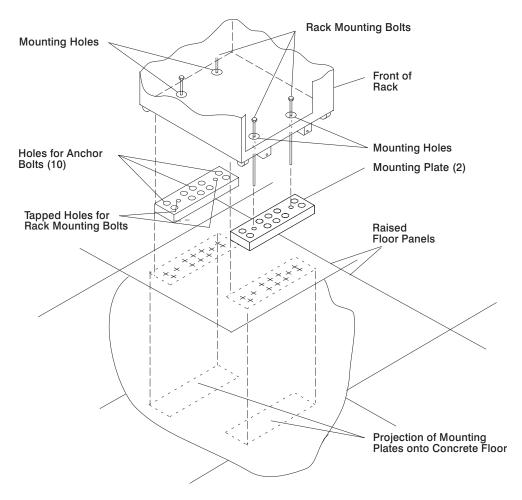
9. At the marked location of the tapped mounting holes, drill two holes approximately 1 inch to allow clearance for the ends of the two rack-mounting bolts. The ends of the rack-mounting bolts may protrude past the thickness of the mounting plate.
