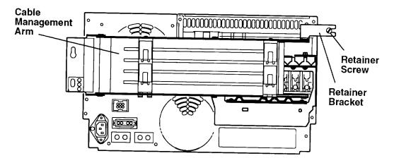
If a retainer bracket is attached to the top of the cable management arm, loosen the screw closest to you and then disengage the bracket from the screw.
