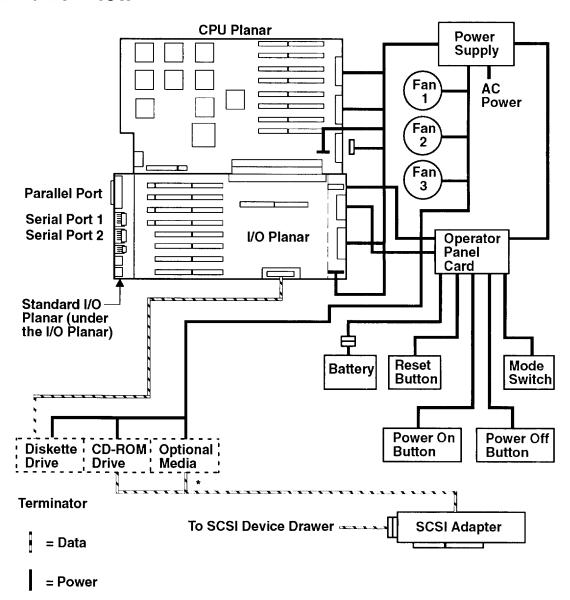
\* The SCSI adapter supplies the data link to all optional media devices except the 5.25-inch diskette drive. The data link for the 5.25-inch diskette drive is supplied by the standard I/O planar.
