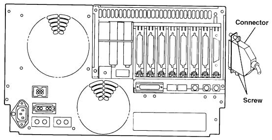
3. Loosen the screw on the strain relief, and then disconnect the device signal cable from the adapter.
