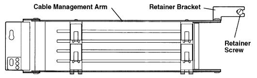
3. If a retainer bracket is attached to the top of the cable management arm, loosen the screw closest to you and then disengage the bracket from the screw.
