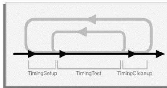
The calls to `timingTest` happen in a tight loop called the *timing loop*. Subclasses or the caller can control how many iterations comprise the timing loop by changing the *timing count*. The total time taken by the timing loop is divided by the number of iterations to get a single *sample time*. The median of all sample times is taken as the estimate of the time to execute the `TimingTest` function.
