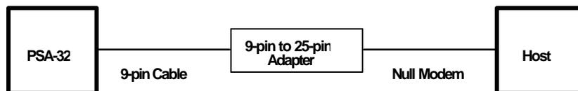
**Figure 3** Typical Serial Connection with an RS-232 UART
