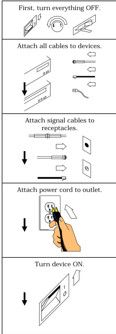
Note: In the UK, by law, the telephone cable must be connected after the power cord.
