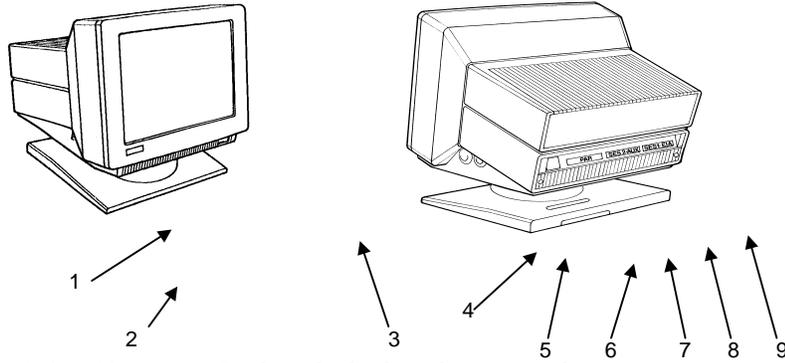
1. Keyboard Connector – Push in the keyboard connector here.
