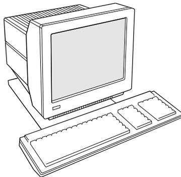
This terminal can emulate a number of ASCII and ANSI terminals, including IBM 3151, PC-Term and SCO™ Console. The keyboards supported by the terminal are the EPC 101-key and EPC 102-key. The dual host capability of the terminal allows you to run two different applications simultaneously. A Setup option is available to view each “session” on the screen in a split or full screen display.
