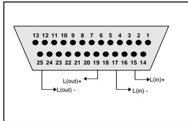
RS-422 Host/Printer Port 1 Pin Assignments
