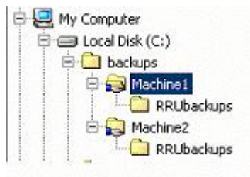
Figure 6. Sample directory tree on a shared network resource set up to receive Rapid Restore Ultra backups
