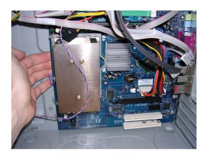
Step 5 (board replacement, if necessary): If a system board is to be replaced, ensure that the system board is properly fit into the chassis. The system board needs to be slid into position such that the CPU retention module slides into the retention clips of the chassis. After sliding the system board (right to left in below picture), lift up on the board to ensure that the board is properly installed. A properly installed board will be securely locked to the chassis wall.
