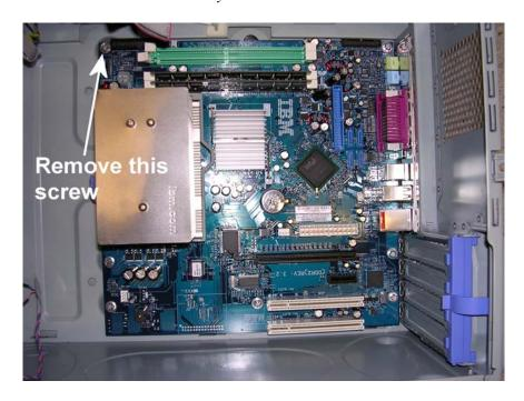
Apply gentle upward pressure under the motherboard near the CPU and heatsink as shown below. Watch the corner of the system board where the screw was removed. If the corner of the board is easily lifted off the screw post, the board was improperly installed and should be replaced. A properly installed board will be locked in place, and not lift off the screw post.
