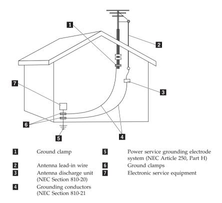
Figure 1. Proper grounding for the cable
