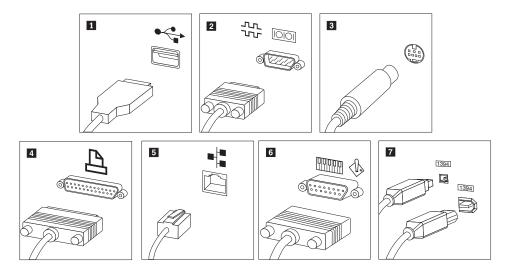
1 USB Use this connector to attach a device that requires a USB connection,
