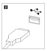
3. Connect the mouse cable to the appropriate keyboard connector, either the standard mouse connector 1 or the USB connector 2.
