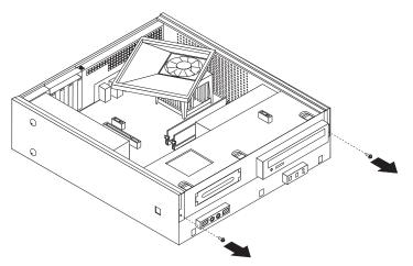
4. Slide the drive bay assembly forward until the drive bay assembly is aligned with the two slots on the sides of the chassis and remove the drive cables from the system board. Then pivot the drive bay assembly upward to remove it completely from the computer.
