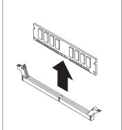
7. Position the replacement memory module over the memory connector. Make sure that the notch 1 on the memory module aligns correctly with the connector key 2 on the system board. Push the memory module straight down into the memory connector until the retaining clips close.
