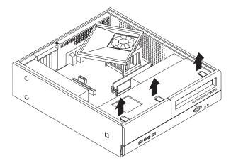
3. Remove the two screws at the front of the chassis securing the drive bay assembly.
