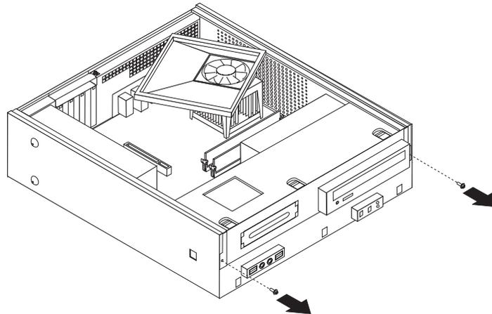
4. In some models, you will need to remove the PCI adapter in order to access the battery.
