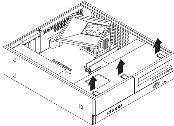
3. Remove the two screws at the front of the chassis securing the drive bay assembly.
