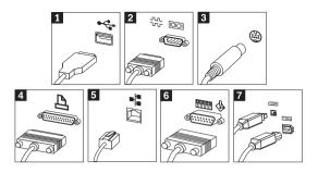
USB Use these connectors to attach a device that requires a Universal Serial Bus (USB) connection, such as a mouse, scanner, printer, or
