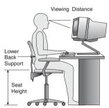
Adjust the monitor so the top of the screen is at, or slightly below, eye level. Place the monitor at a comfortable viewing distance, usually 51 to 61 cm (20 to 24 in.), and position it so you can view it without having to twist your body. Also position other equipment you use regularly, such as the telephone or a mouse, within easy reach.
