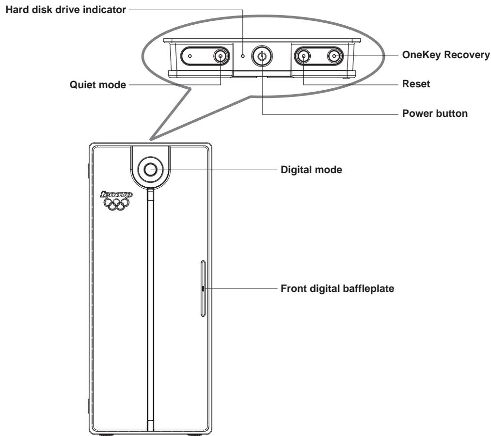
**Power button:** By pressing this key, you can start up or shut down the computer.
