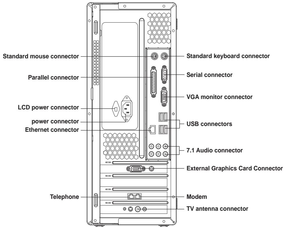
**power connector:** Used to supply power to the computer.
