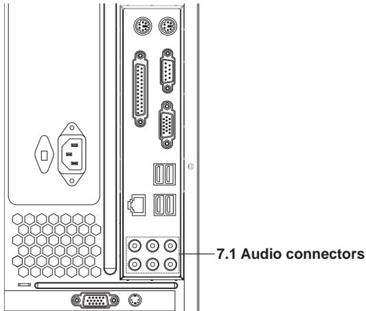
**7.1 Audio connectors:** audio input, microphone, line out, rear speaker output, central/ heavy bass output, side speaker output.
