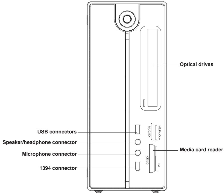
**USB connectors:** Used to connect USB devices.
