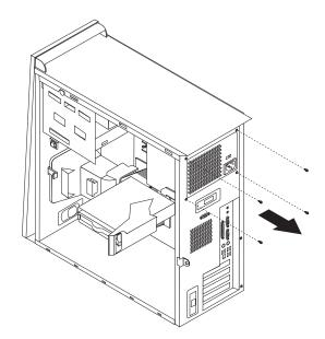
6. Press inward on the metal retainer and remove the power supply from the computer.
