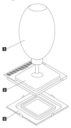
• If you are installing a microprocessor from the old system board to a new system board, use the vacuum pen 1 to pick up the microprocessor.
