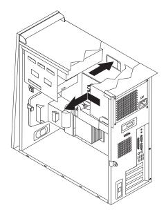
7. Install the new power supply into the chassis so that the screw holes in the power supply align with those in the chassis.
