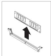
4. Make sure the DIMM notch 1 aligns correctly with the connector key 2 on the system board. Push or insert the DIMM straight down into the connector until the retaining clips close.
