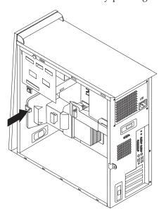
5. Disconnect the fan cable from the system board. Note the cable location on the system board.
