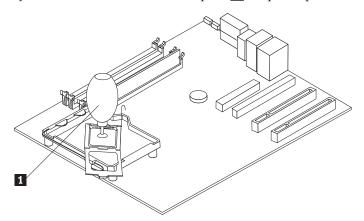
10. Notice of the orientation of the notches 1 in the microprocessor. This is important when reinstalling the microprocessor on the system board.
