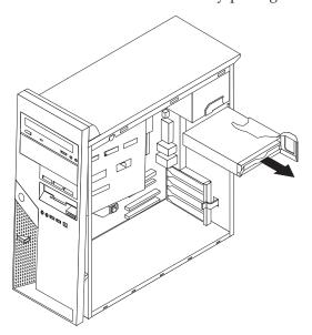
5. Remove the drive from the blue bracket by flexing the bracket.
