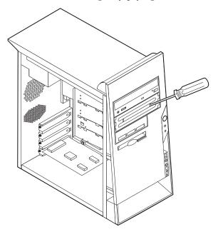
5. Make sure the drive that you are installing is set correctly as either a master or a slave device.
