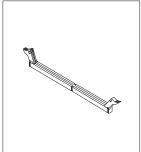
5. Make sure the notches in the DIMM align with the tabs on the connector. Push or insert the DIMM straight down into the connector until the retaining clips close.
