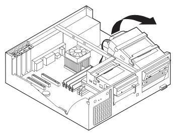
6. Make sure the drive that you are installing is set correctly as either a master or a slave device.
