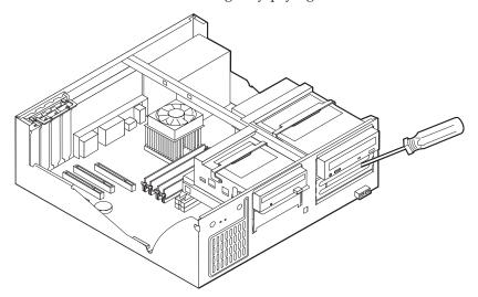
5. Pivot the drive-bay latch handle toward the front of the computer and then pivot the drive-bay cage upward, as shown, until it is latched in the upright position.
