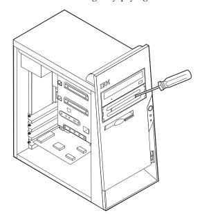
5. Make sure the drive that you are installing is set correctly as either a master or a slave device.
