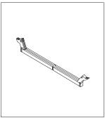
4. Make sure the notch in the DIMM aligns with the tab on the connector. Push or insert the memory module straight down into the connector until the retaining clips close.
