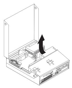
4. If any PCI adapters are installed, remove the PCI riser and adapter cards. Do not remove any adapters from the riser card. See "Installing PCI adapters" on page 17.
