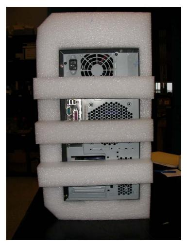
2.9 - Place the cushioned unit into the bottom of the carton, making sure the handholds are on the top and bottom of the system. Improper loading of the system will reneder the handholds useless.
