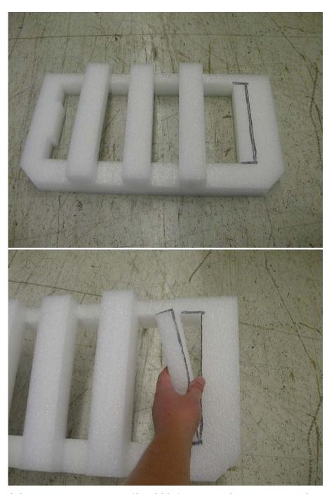
2.8 - Place the cushions (37L8095) over the front and rear of the bagged machine (the bag has been removed from all pictures for clarity).
