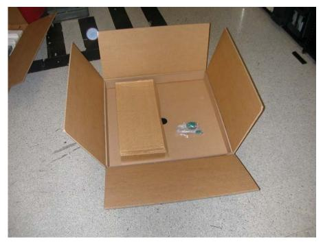
2.16 - Bend the top four flaps of the CPU carton inward (minor flap inside major flaps) so the scores are broken. Send the assembly down the conveyor to be sealed using IBM logo tape (74F5699).
