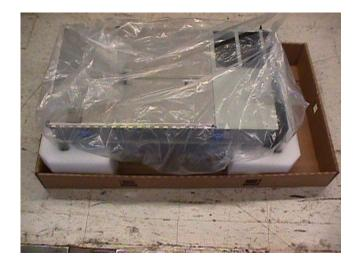
**2.9** Use **01R3747** to tape lift handle position sheet **24P1226** to top cover in approximate position as shown. Do not place tape over labels.
