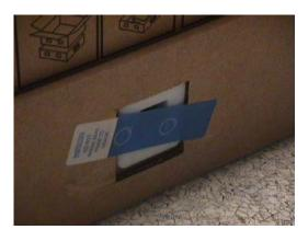
2.15 Place divider (25P1144) in front of the machine with knock down tab
