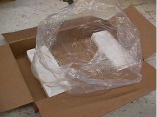
**2.6** - Place the machine inside the bag on the cushions. The second picture does not have a bag
