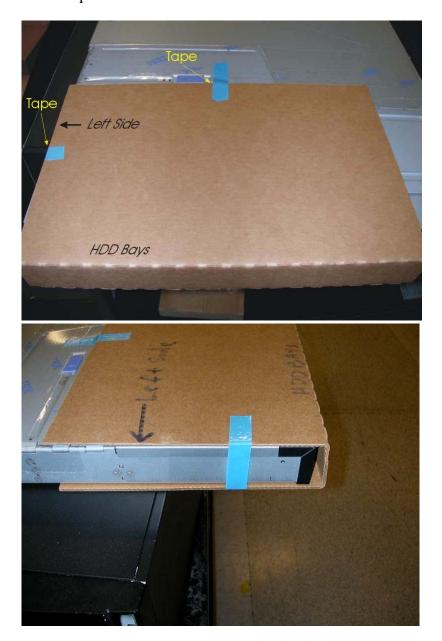
1.3 - Assemble carton 39Y7687 and tape the bottom flaps shut with IBM Logo Tape 74F5698 or 74F5699. **Note: Old version artwork on carton is depicted.**
