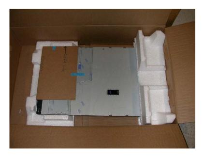
1.8 - Place front top half of cushion down in front of system, and then slide it back into position next to the HDDs. **Take great care not to force cushion downward as damage may occur.**
