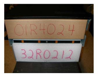
2.8 Place unit in bottom cushions. Make sure system in positioned all the way down and not sitting on the cushion ledge. Pull the bag up around the sides of the unit and fold neatly on top.
