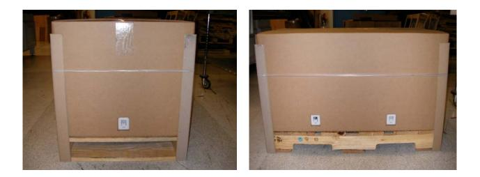
3.2 Place one 24 inch corner board on each of the two short top edges of the package and two way band the unit to the half-pallet.
