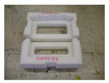
2.5 Place bottom front cushion (01R4043) in tray. Make sure bottom front cushion is placed in tray so the side cutouts on the cushion align with front, side clip holes in tray and leave approximately 4.5 inches of space between the front cushion and front edge of bottom tray. Place bottom rear cushion (01R4044) all the way to the back of the tray.
