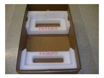
2.6 Place bag (37L0557) over bottom cushions and pull bag down around sides of bottom tray in preparation for loading unit.
