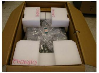
2.17 Place rail kit in center cavity between the top cushions. The rail kit should nest inside the top cushions. Make sure the kit is pushed all the way down and sits below the surface of the top cushion.
