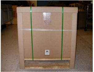
3.3 Stretch wrap the unit to the pallet utilizing Best of Breed" methods. The Stretch wrapping Machine MUST wrap a minimum of three times around the base and four times around the top of the load with 100% coverage of the product using the roping technique. If roping capabilities are not available you Must use palletization Methods 2 or 3 as outlined in documents 92F6168 "Best of Breed" Pallet Unitization or QMX document P-04146.
